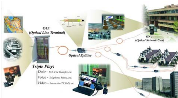
Fig. 12 Fiber-To-The-Home (FTTH) architecture and services
