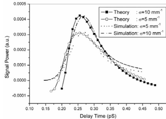
Fig. 2. Temporal evolution of reflectance calculated by using BEM (dash line) and Theoretical method with different value of scattering coefficient (other lines).
