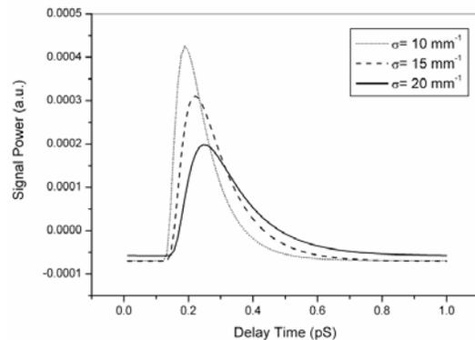
Fig 3. Effect of scattering coefficient on reflected pulse.
