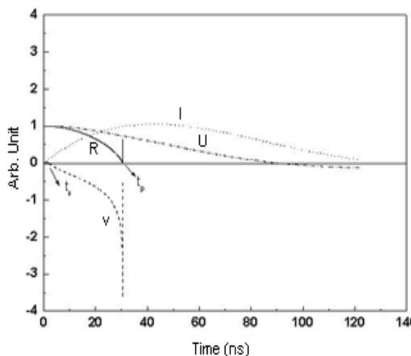
**Fig. 2:** Time dependencies of normalized radius  $\chi$ , velocity  $v$ , current  $I'$  and voltage  $\eta$  for  $\alpha = 1.5748 \times 10^5$ ,  $\beta = 0.2543$ , and  $\gamma = 0.5401$  (Voltage=400 kV, current peak=32 kA, period=220 ns Capillary radius=1.5 mm)
