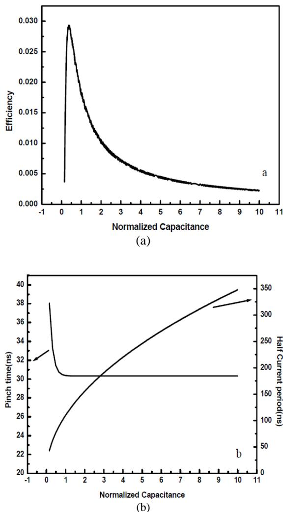
**Fig. 4:** Dependencies of (a) efficiency and (b) pinch time and half current period on normalized capacitance  $\kappa$  for  $\alpha=1.5748 \times 10^{-5}$ ,  $\beta=0.2543/\kappa$ , and  $\gamma=0.5401$
