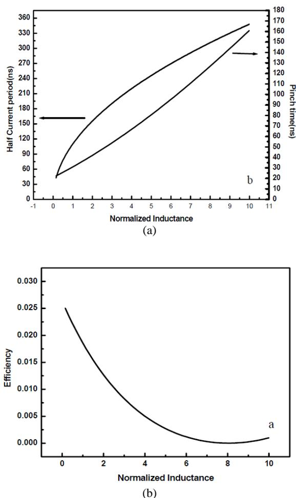
**Fig. 3:** Dependencies of (a) efficiency and (b) pinch time and Half Current period on Normalized Inductance,  $\sigma$ , for  $\alpha=1.5748 \times 10^{-5} \sigma$ ,  $\beta=0.2543$ ,  $\gamma=0.5401/\sqrt{\sigma}$  (Voltage=400 kV, Current peak=32 kA, Current period=220 ns, Capillary radius=1.5 mm)
