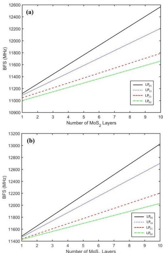
Fig. 8. Investigation of the effect of different layers MoS<sub>2</sub> on the BFS as a function of temperature and strain for 4 modes at (a) 100 °C and (b) 8000 με.
