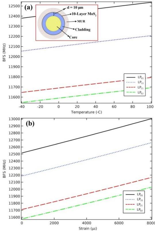
Fig. 7. Relationship between BFS and (a) temperature and (b) strain at the wavelength of 1550 nm for 10-layer MoS<sub>2</sub>.
