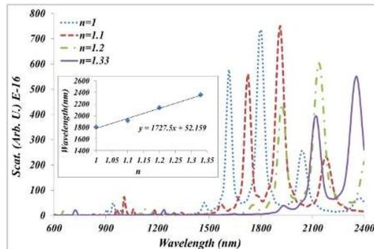
Fig. 7. Scattering cross-sections of SHS with number of steps=3 and structure radius  $r=5\text{ nm}$  under normal incidence light for various refractive index from 1 to 1.33. Inset: The wavelength of LSPR peaks Vs. the refractive index of the surrounding medium.
