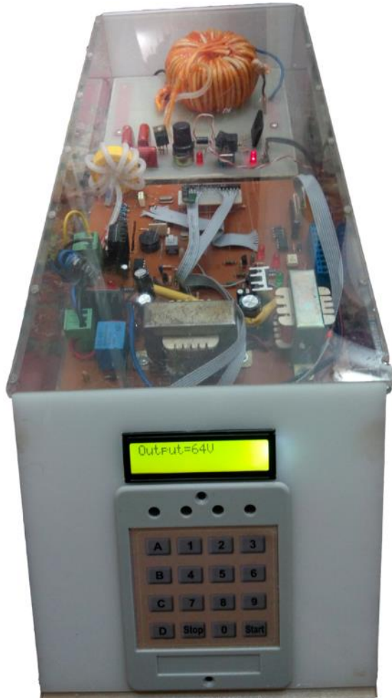
Fig. 1. A view of home-made pulsed light driver
