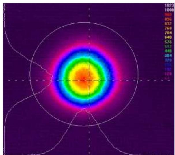
Fig. 9. Far field profile of generated 532 nm lights.
