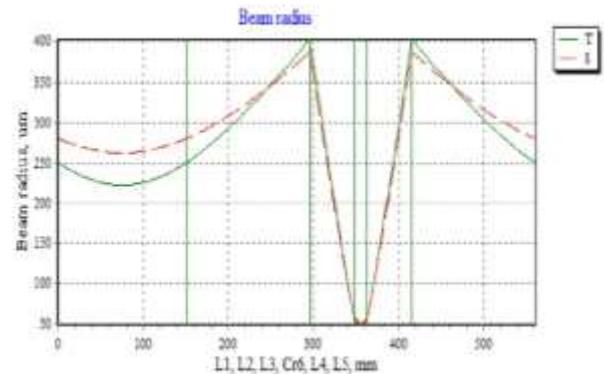
Fig. 2. Beam radius along the designed enhancement cavity
