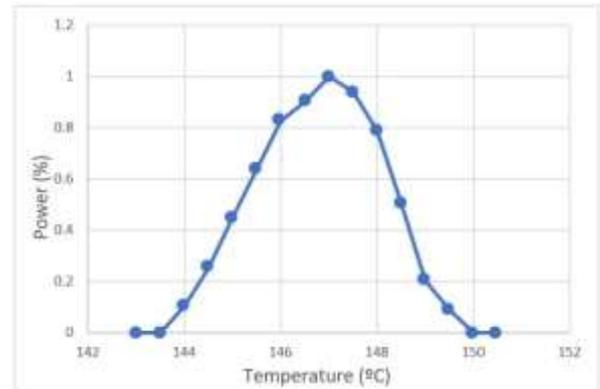
Fig. 8. Phase matching diagram of the noncritical phase matched, 15mm LBO crystal.
