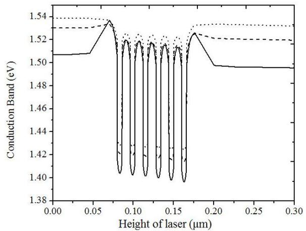
Fig. 6. Conduction Band near the laser axis for different p- doping level (solid: no doping, dashed:  $2 \times 10^{17} \text{ cm}^{-3}$ , dotted:  $2 \times 10^{18} \text{ cm}^{-3}$ ) at an injection current of 90 mA and a stage temperature of 80°C.
