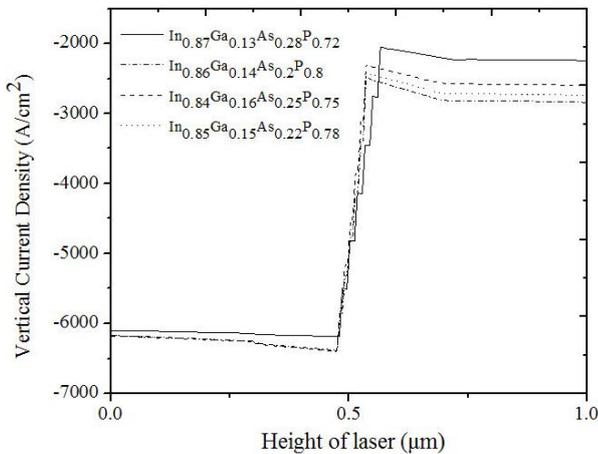
Fig. 17. Vertical Current Density of electrons near the laser axis for different barrier layer at an injection current of 90 mA and a stage temperature of 80°C.
