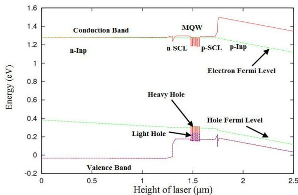
Fig. 2. Energy band diagram at 30 mA ( $T=80^\circ\text{C}$ ).
