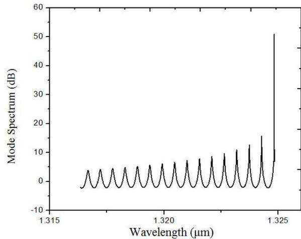
Fig. 18. Laser mode spectrum with tensile barrier at 90 mA ( $T=80^{\circ}\text{C}$ ).
