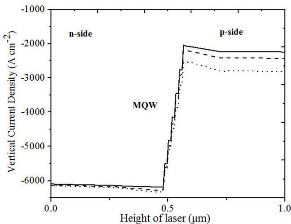
Fig. 5. Vertical current density of electrons near the laser axis for different p- doping level (solid: no doping, dashed:  $2 \times 10^{17} \text{ cm}^{-3}$ , dotted:  $2 \times 10^{18} \text{ cm}^{-3}$ ) at an injection current of 90 mA and a stage temperature of 80°C.
