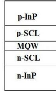
Fig. 1. The structure of the studied laser.
