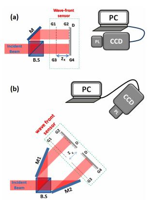
Fig. **4** Schematic of two different arrangements of two-channel moiré based wavefront sensor: B.S is beam splitter, M, M1, M2 are mirrors, G1-G4 are Ronchi gratings and P1 is collimated lens that projects the moiré pattern produced on the diffuser D on the CCD camera.
