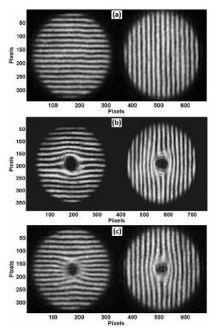
Fig. **5** Typical recorded frames of moiré patterns for three different cases of the incident beam: (a): plane wave, (b): vortex beam, recorded by the set-up of Fig. 4(a), (c): same beam by the set-up of Fig. 4(b).
