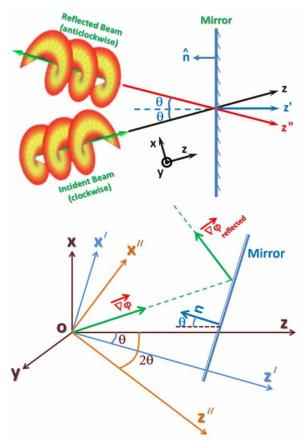
Fig. **1** Representation of a typical incident and reflected vortex beam from a mirror and all of the selected coordinate systems.
