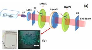
Fig. **3** (a): Schematic of the experimental setup is used for generation of the LG beam from a q-plate: SF is spatial filter, P1, P2 are polarizers, and QWP1 and QWP2 are the first and second quarter-wave plates, (b): left: q-plate, right: q-plate between two crossed polarizers.
