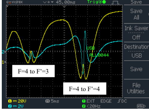
Fig. 5. Experimental results of the \sigma absorption lines (yellow traces), and the sub-Doppler error signal (blue trace).
