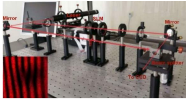
Fig. 6 Mach-Zehnder interferometer setup, the fork grating is obtained from Mach-Zehnder which shows the topological charge one ( l=1 ).
