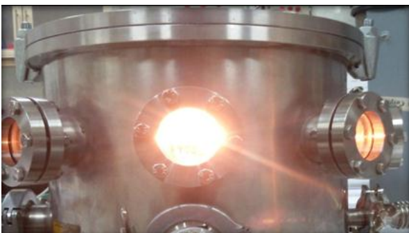
Fig. 1. The HFCVD system in the real experiment condition for synthesis of NCD film.
