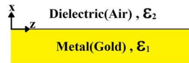
Fig. 1. Geometry of a metal-dielectric junction for the movement of surface plasmon polaritons. ( \epsilon_1 = -877 + 610i and \epsilon_2 = 1 )
