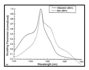
Fig. 10 The fluorescent spectrum of a sample EDFA.
