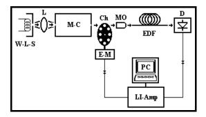
Fig. 7 Experimental setup for measurement of EDF absorption spectrum. WL-S: white light source, L: lens, M-C: monochromator, Ch: chopper, E-M: chopper electro-motor, MO: microscope objective, EDF: erbium-doped fiber, LI-Amp: lock-in amplifier, PC: personal computer, D: optical detector. The setup can be modified to swap the monochromator by an optical spectrum analyzer (OSA) [1].
