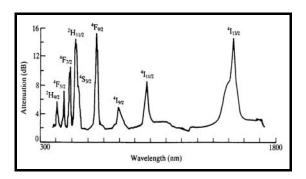
**Fig. 8** Absorption spectrum of a sample EDFA [28].
