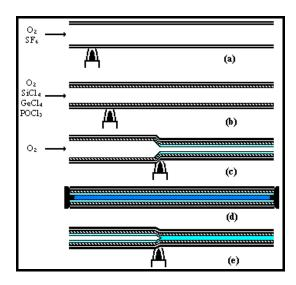
**Fig. 1** Preform fabrication by MCVD method and Er incorporation by solution doping, (a) cleaning and drying the tube, (b) cladding and core depositions, (c) partial collapse, (d) solution doping, and (e) collapse process [1].
