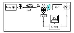
Fig. 9 Experimental setup for measurement of fluorescent spectrum. Pump: 514.5 nm argon laser, 980 nm, or 1480 nm laser diode, MO: microscope objective, SMF: single mode fiber, EDF: erbiumdoped fiber, Ch: chopper, E-M: chopper electromotor, F: pump rejection filter. M-C: monochromator, **D**: optical detector, LI-Amp: lock-in amplifier, PC: personal computer. The setup can be modified to swap the monochromator by an optical spectrum analyzer (OSA) [1].
