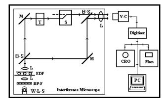
Fig. 5 Setup for fiber refractive index measurement by the interferometry method. W-L-S: white light source, BP-F: 598 nm band pass filter L: lens, EDF: erbium-doped fiber at the center, B-S: beam splitter, M: mirror, T: tilter, S: shifter, V-C: video camera, CRO: cathode ray oscilloscope, PC: personal computer, Mon: monitor [1].
