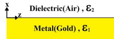
Fig. 1. Geometry of a metal-dielectric junction for the movement of surface plasmon polaritons. ( \epsilon_1 = -877 + 610i and \epsilon_2 = 1 )
