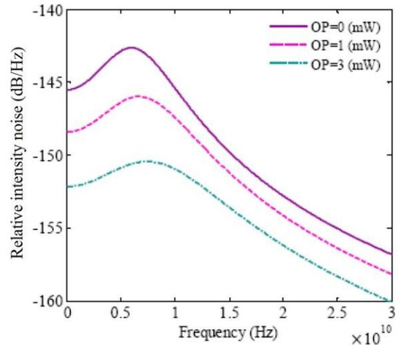
Fig. 8 The relative intensity noise spectrum of InAs/InP QD laser for three different values of optical pumping and at the injection current of  $I=55\text{mA}$ . External optical beam decreases the level of RIN and increases the damping factor.
