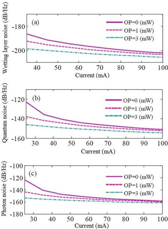
Fig. 9 The values of the (a) WL, (b) quantum, and (c) photon noises versus current at  $f=1\text{GHz}$  for three different optical pump powers. External optical beam reduces the values of three shot noise sources at all bias points.
