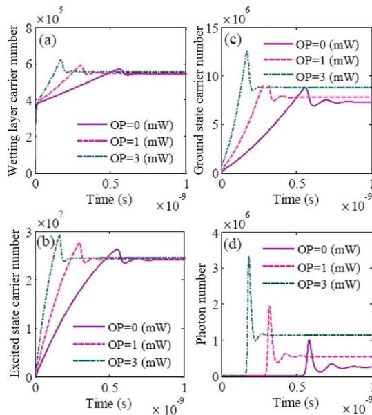
Fig. 6 Turn-on dynamics of carriers and photons for a step current from zero to  $I=55\text{mA}$ . The number of carriers at all three states of the (a) WL, (b) ES, and (c) GS and also (d) photons grow during shorter delay time by increasing the external optical pump.
