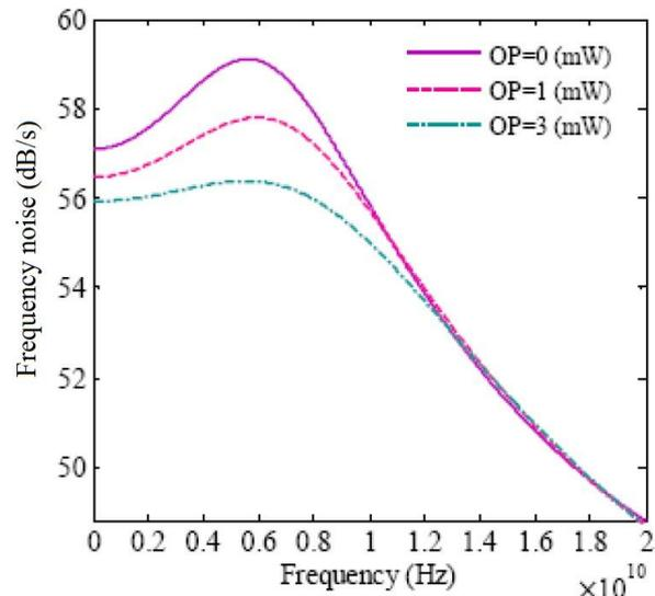
Fig. 11 The frequency noise spectrum of QD laser for three different optical pump powers and at the injection current of  $I=55\text{mA}$ . The FN level reduces and the resonant frequency grows at higher optical pumps.
