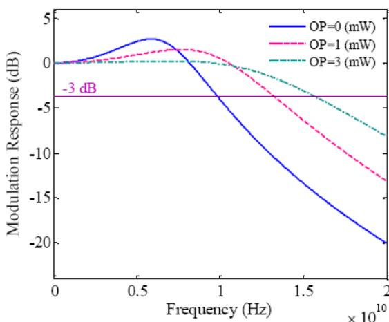
Fig. 4 Modulation response of QD laser for three different values of optical pumping and at  $I=55\text{mA}$ . Optical pump makes the modulation response of QD laser wider and increases its 3dB bandwidth.
