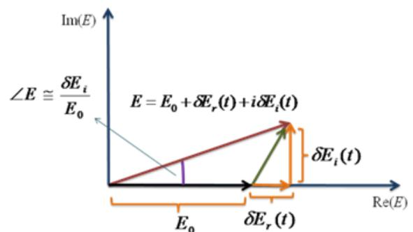
Fig. 2 Vector illustration of the relationship between the instantaneous field magnitude and the in-phase and out-phase noise components [25].
