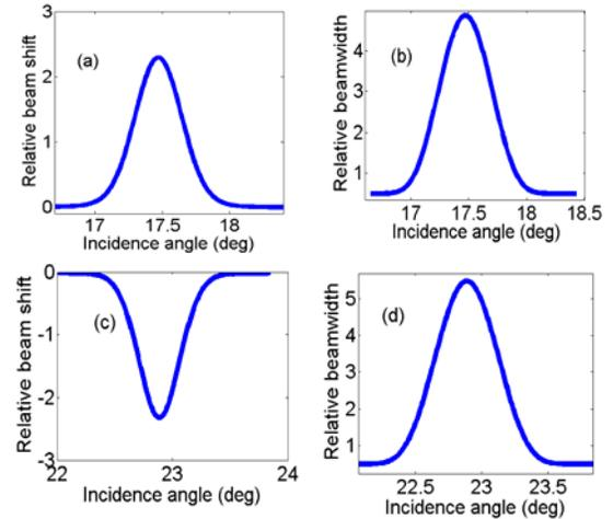
**Fig. 3** Relative beam shift and beam width versus the incidence angle corresponding to forward (a), (b) and backward (c), (d) surface states. Here  $L = 3.6 \text{ cm}$  for (a), (b) and  $L = 2.12 \text{ cm}$  for (c), (d).
