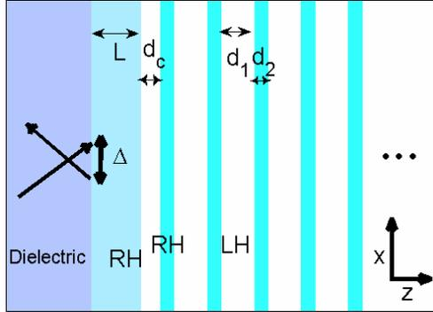
**Fig. 1** Geometry of the problem. In our calculations, we take the following values:  $d_1 = 2.5 \text{ cm}$ ,  $d_2 = 1 \text{ cm}$ ,  $d_c = 0.6d_1$ ,  $n_0 = 3.5$ ,  $\mu_0 = 1$ ,  $n_1 = -2$ ,  $\mu_1 = -1$ ,  $n_2 = 1.5$ ,  $\mu_2 = 1$ ,  $n_R = 1$ ,  $\mu_R = 1$ .
