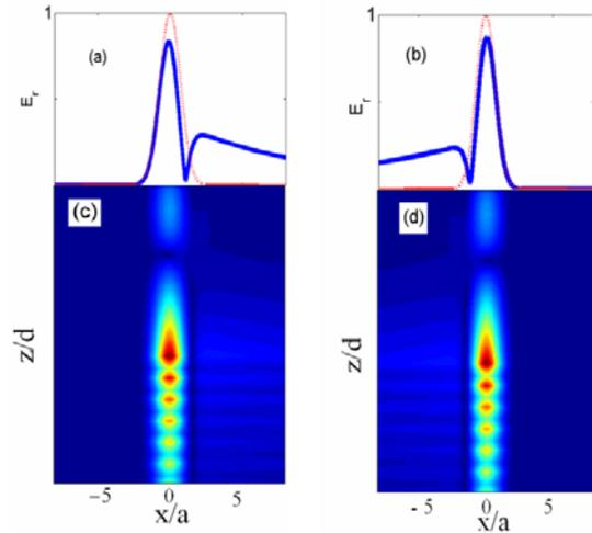
**Fig. 5** Profiles of the reflected (solid) and incident (dotted) beams shown as the field amplitude versus coordinate  $x$  for incidence angle of beam (a)  $\theta = 17.45^\circ$  in the case forward surface state (b)  $\theta = 22.86^\circ$  in the case backward surface state. Field distribution of the surface states are shown in (c) and (d) corresponding to (a) and (b). Here  $d = d_1 + d_2$ .
