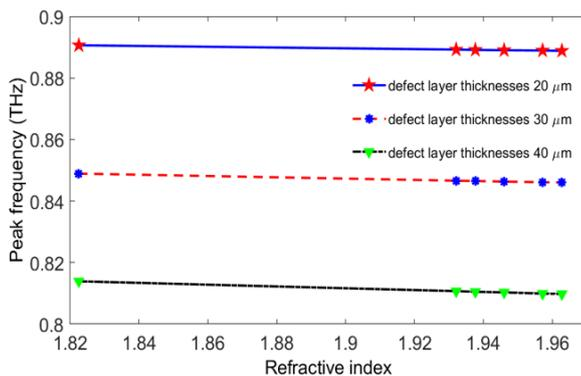
Fig. 10. The peak frequency of the defect modes of the 1D-PC-based biosensor with the structure  $(AB)^5D(AB)^5$  versus the refractive index,  $n$ , of the analyte cancer cells for different thicknesses of the defect layer. The other parameters used here are the same as in Fig. 3.
