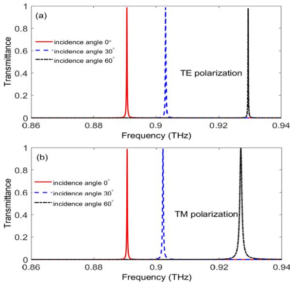
Fig. 3. The transmittance of the 1D-PC-based biosensor with the structure  $(AB)^5D(AB)^5$  versus the frequency  $f$  for a) the TE-polarized and b) the TM-polarized incident waves at three different incidence angles  $\theta$ . Here, we assumed that the defect layer  $D$  with the thickness  $d_D=20 \mu m$  is filled with the normal cells, and the other parameters are the same as in Fig. 2.
