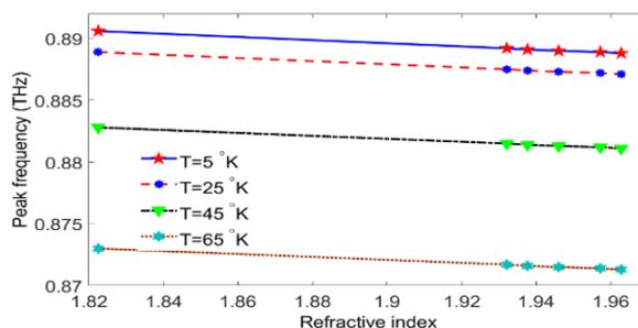
Fig. 7. The peak frequency of the defect modes of the 1D-PC-based biosensor with the structure  $(AB)^5D(AB)^5$  versus the refractive index  $n$ , of the analyte cancer cells at different temperature  $T$ . The other parameters used here are the same as in Fig. 3.
