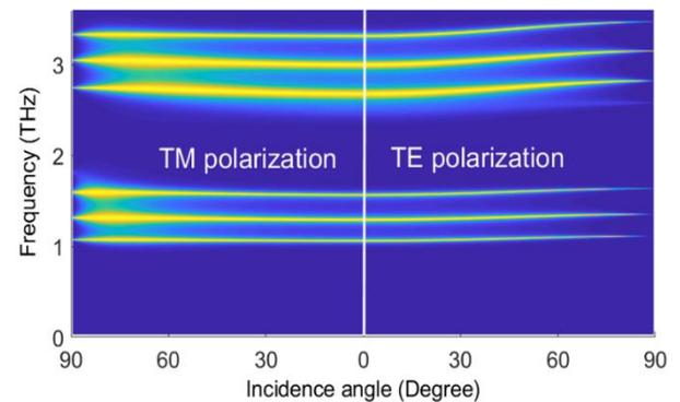
Fig. 2. The transmittance of the 1D-PC with the structure  $(AB)^5$  in the plane  $(f, \theta)$ . Here,  $d_A = 5 \mu\text{m}$ ,  $d_{0B} = 20 \mu\text{m}$ ,  $T = 4.2 \text{ K}$ , and  $P = 1 \text{ atm}$ .
