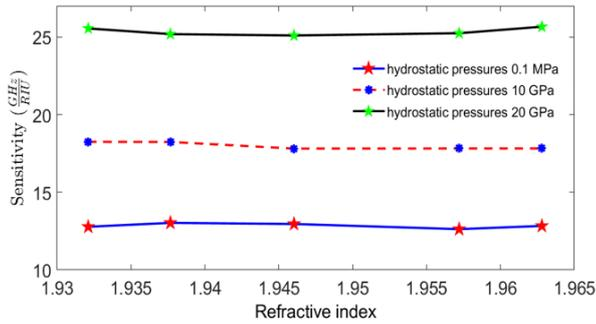
Fig. 9. The sensitivity ( $S$ ) of the 1D-PC-based biosensor with the structure  $(AB)^5D(AB)^5$  versus the refractive index,  $n$ , of the analyte cancer cells at different hydrostatic pressures  $p$ . The other parameters used here are the same as in Fig. 3.
