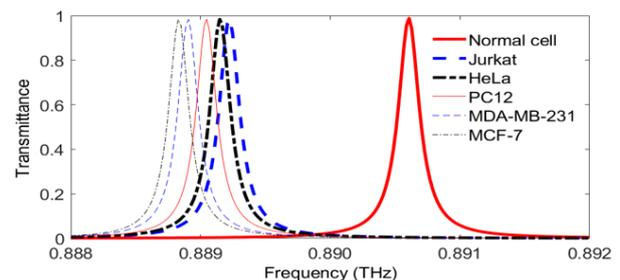
Fig. 5. The transmittance of the 1D-PC-based biosensor with the structure  $(AB)^5D(AB)^5$  versus the frequency  $f$  at the incidence angle  $\theta=0$  for various analyte types (normal cells (the thick solid line), Jurkat (the thick dashed line), HeLa (the thick dash-dot line), PC12 (the thin solid line), MDA-MB-231 (the thin dashed line), MCF-7 (the thin dash-dot line)). The other parameters used here are the same as in Fig. 3.
