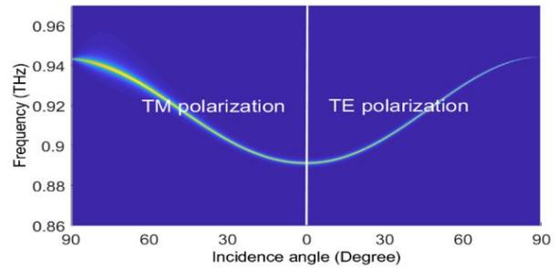
Fig. 4. The transmittance of the 1D-PC-based sensor with the structure  $(AB)^5D(AB)^5$  in the plane  $(f, \theta)$ . The parameters used here are the same as in Fig. 3.
