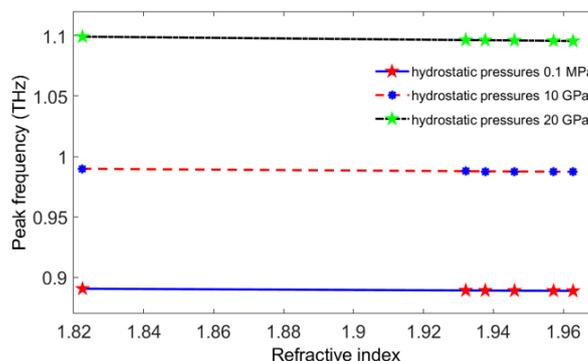
Fig. 8. The peak frequency of the defect modes of the 1D-PC-based biosensor with the structure  $(AB)^5D(AB)^5$  versus the refractive index,  $n$ , of the analyte cancer cells at different hydrostatic pressures  $P$ . The other parameters used here are the same as in Fig. 3.
