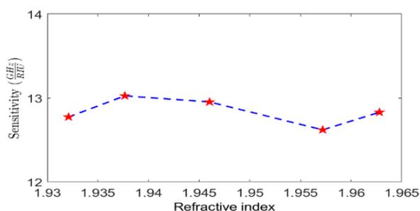
Fig. 6. The sensitivity ( $S$ ) of the 1D-PC-based biosensor with the structure  $(AB)^5D(AB)^5$  versus the refractive index,  $n$ , of the analyte cancer cells. The parameters used here are the same as in Fig. 3.
