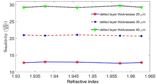
Fig. 11. The sensitivity ( $S$ ) of the 1D-PC-based biosensor with the structure  $(AB)^5D(AB)^5$  versus the refractive index,  $n$ , of the analyte cancer cells for different thicknesses of the defect layer. The other parameters used here are the same as in Fig. 3.
