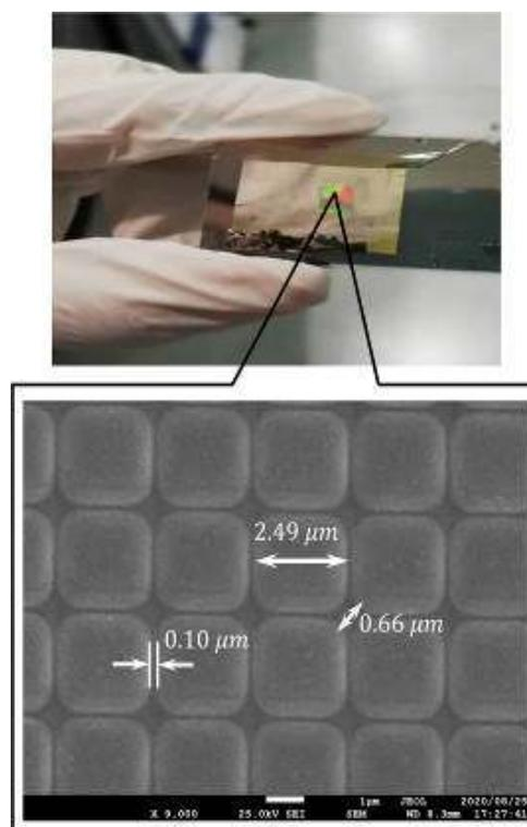
Fig. 2. SEM image of the fabricated plasmonic crystal.
