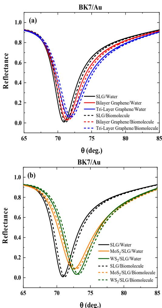
Fig. 2. SPR reflectance curves for (a) SLG, bilayer graphene, trilayer graphene, and (b) WS<sub>2</sub>/SLG and MoS<sub>2</sub>/SLG structures in water and biomolecules medium on the BK7/Au substrate.
