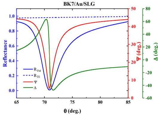
Fig. 3. Reflectance of TM (solid blue line) and TE (blue dashed line) light,  $\Psi$  (red), and  $\Delta$  (olive) for BK7/Au/SLG. Orange vertical line shows that in resonance angle abrupt change in phase occurs.
