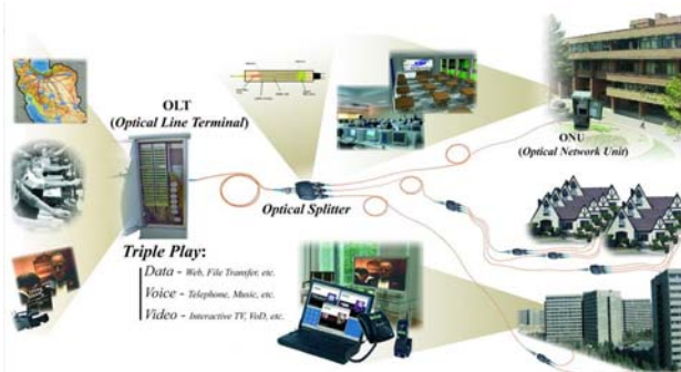
Fig. 12 Fiber-To-The-Home (FTTH) architecture and services
