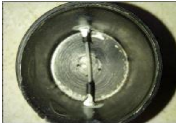
Fig. 2. Photograph of tapered portion and uniform core portion surface of the fiber.
