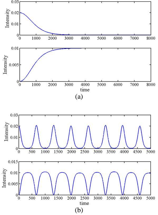
Fig. 1 Time evolution of the intensities  $|a|^2$  (top panel) and  $|b|^2$  (bottom panel) vs. electric field  $\varepsilon$ . (a) steady-state response ( $\varepsilon = 0$ ), (b) pulsing behavior ( $\varepsilon = 10^{-6}$ ).
