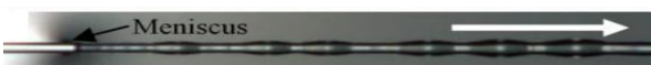
Fig. 2: the picture shows the micro-droplets distribution along the fiber caused by surface tension via stretching of the fiber [7].
