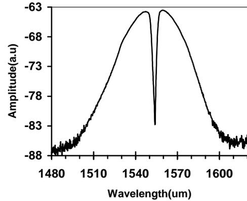
Fig. 3 Frequency response of a 1-D grating structure.
