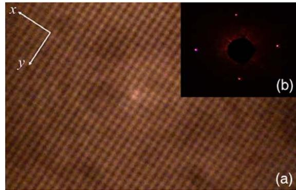
**Fig. 5** photograph of an actual fabricated 2-D rectangular structure, as observed under polarizing microscope. The inset shows the diffraction pattern of this photonic crystal obtained exposing the PC to a HeNe laser.
