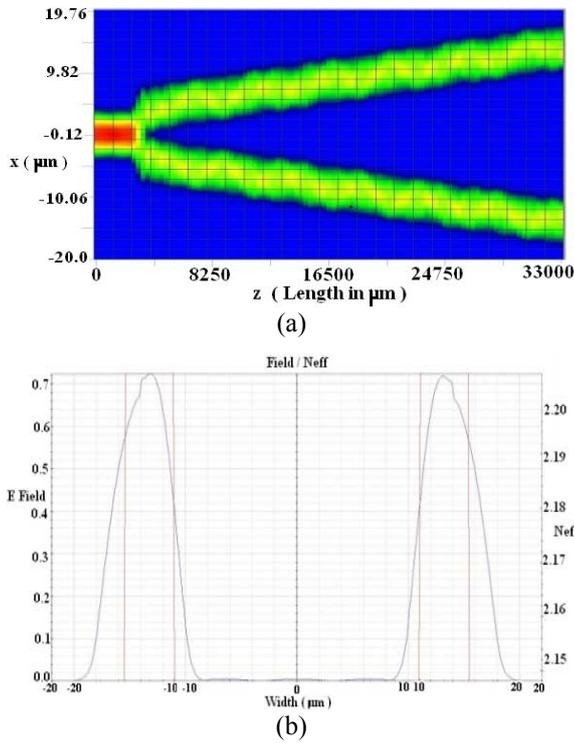
**Fig. 4** Operation at 1.55  $\mu\text{m}$  optical power input (a) Optical Field propagation in the DOS architecture (b) cut view of the output section, graph showing electric field intensity (curved shaped) and refractive index distribution (rectangular shaped) over the section.
