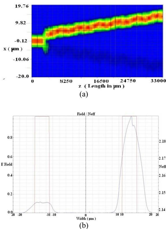
**Fig. 7** Operation at 1.55  $\mu\text{m}$  optical powers input with -24 V bias on middle electrode. (a) Optical field propagation in the DOS architecture (b) cut view of the output section, graph showing electric field intensity (curved shaped) and refractive index distribution (rectangular shaped) over the section.
