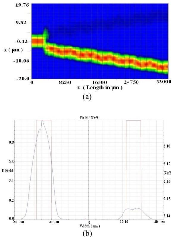
**Fig. 6** Operation at 1.55  $\mu\text{m}$  optical powers input with +24 V bias on middle electrode. (a) Optical field propagation in the DOS architecture (b) cut view of the output section, graph showing electric field intensity (curved shaped) and refractive index distribution (rectangular shaped) over the section.
