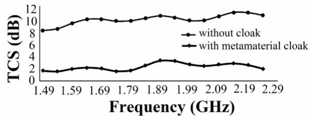
Fig. 3 Total scattering of cloaked and un-cloaked PEC shell with metamaterial in various frequencies.
