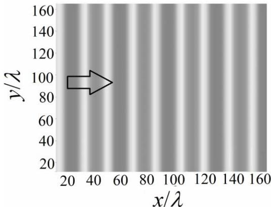
Fig. 2  $H_z$  distribution of  $TE_z$  plane-wave propagating along x-direction, with applying the CPML boundaries conditions
