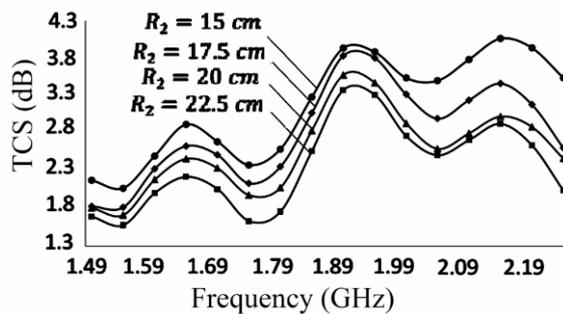
Fig. 5 total scattering of cloaked PEC with different thicknesses in various frequencies
