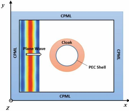
Fig. 1 Calculation scheme for cylindrical cloak structure with PEC core and CPML boundaries conditions
