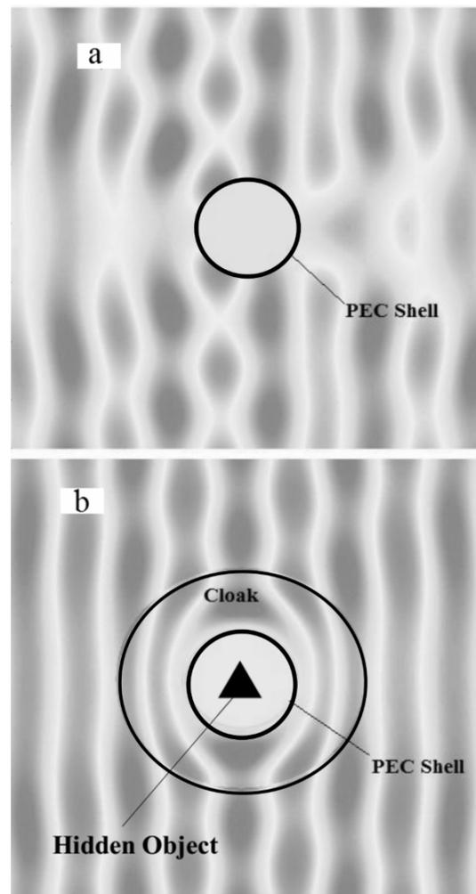
Fig. 4  $H_z$  distribution of wave around a) PEC Shell and b) coated PEC shell by ideal metamaterial cloak.
