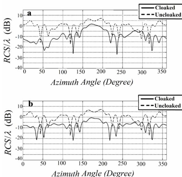
Fig. 6 RCS diagram of bare and cloaked with metamaterial PEC with a)  $t=5$  cm b)  $t=12.5$  cm, thicknesses in 1.55 GHz
