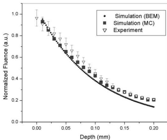
Fig. 4. Calculated normalized fluence by MC and Green theorem based on Green method for different depths and compared with experimental value of depths.
