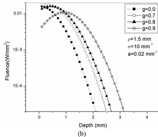
Fig. 2. The simulated fluence at different distance from location of illumination of laser for several value of anisotropic factor. (a) at distance of  $\rho = 0.5$  mm and (b)  $\rho = 1.5$  mm
