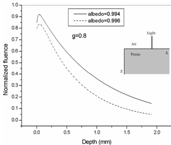
Fig. 1. The estimated fluence of penetrating photons inside biological phantom for different values of albedo.
