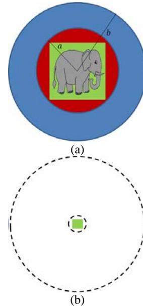
Fig. 1. A schematic diagram for the illusion device. (a) Physical space: a large object (elephant) is inserted in a box and the box is placed in the core of the device. (b) Virtual space: the observer sees a box (matchbox) that is much smaller than the real box in physical space and the object inside. The object is not visible.
