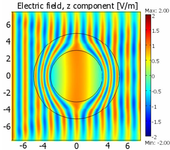
Fig. 2. Full wave simulation of the z-component of the electric field for a TE plane wave with  $a = 2\lambda = 2$ ,  $b = 5$  and  $c = 0.5$  incident on the empty illusion device.
