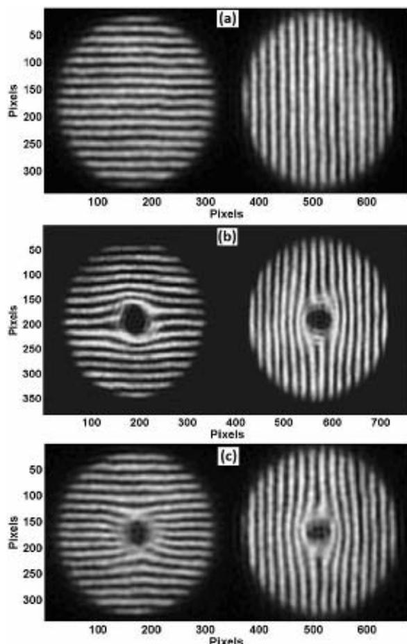
Fig. 5 Typical recorded frames of moiré patterns for three different cases of the incident beam: (a): plane wave, (b): vortex beam, recorded by the set-up of Fig. 4(a), (c): same beam by the set-up of Fig. 4(b).
