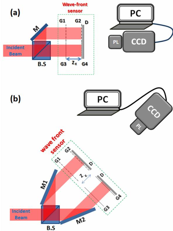
Fig. 4 Schematic of two different arrangements of two-channel moiré based wavefront sensor: B.S is beam splitter, M, M1, M2 are mirrors, G1-G4 are Ronchi gratings and PL is collimated lens that projects the moiré pattern produced on the diffuser D on the CCD camera.
