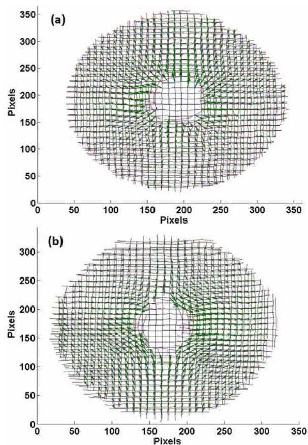
Fig. 6 Two-dimensional diagrams of the displacement vectors of the moiré patterns corresponding to the moiré patterns of (a): Fig. 5(b) and (b): Fig. 5(c).
