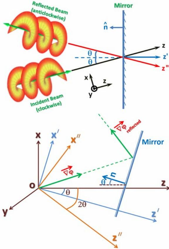
Fig. 1 Representation of a typical incident and reflected vortex beam from a mirror and all of the selected coordinate systems.
