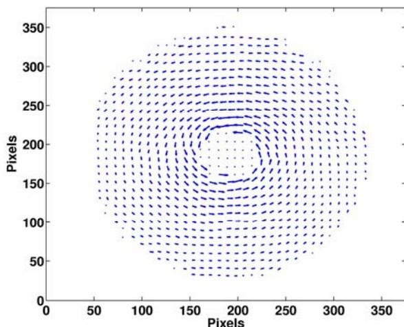
Fig. 7 Diagram of the calculated gradients vectors for LG cross section for  $l=20$ .
