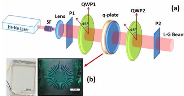
Fig. 3 (a): Schematic of the experimental setup is used for generation of the LG beam from a q-plate: SF is spatial filter, P1, P2 are polarizers, and QWP1 and QWP2 are the first and second quarter-wave plates, (b): left: q-plate, right: q-plate between two crossed polarizers.
