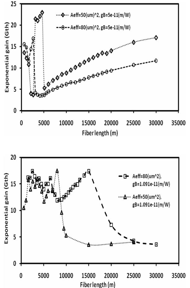
Fig. 9  $G_{th}$  vs. fiber length corresponding to different kinds of  $A_{eff}$  and  $g_B$ .
