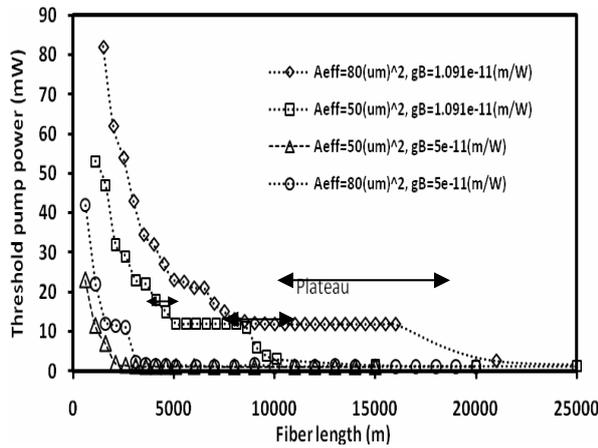
Fig. 8 Threshold pump power vs. fiber length, corresponding to different values of  $A_{eff}$  and  $g_B$  using 1% criterion.
