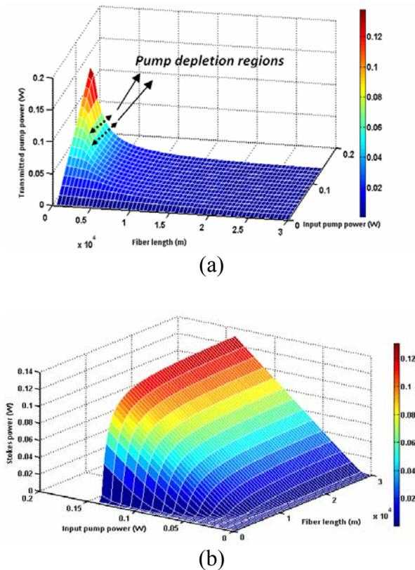
Fig. 6 Transmitted pump (a) and Stokes power (b) vs. input pump power for different fiber lengths.
