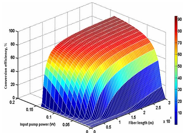
Fig. 7 Conversion efficiency vs. input pump power for different lengths of fiber.
