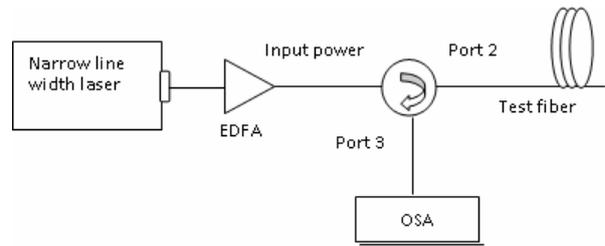
Fig. 2. The experimental configuration to measure SBS power threshold.
