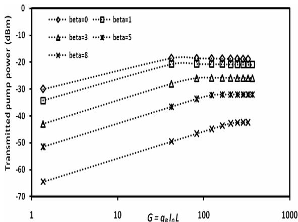
Fig. 4. Transmitted pump power vs. gain  $G = g_B I_0 L$  for different fiber loss.
