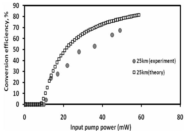
Fig. 3. Conversion efficiency obtained by the theoretical and experimental results Vs. input pump power.
