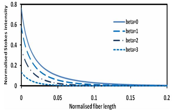
Fig. 1. Normalized transmitted pump and Stokes intensities vs. fiber length for different fiber loss.
